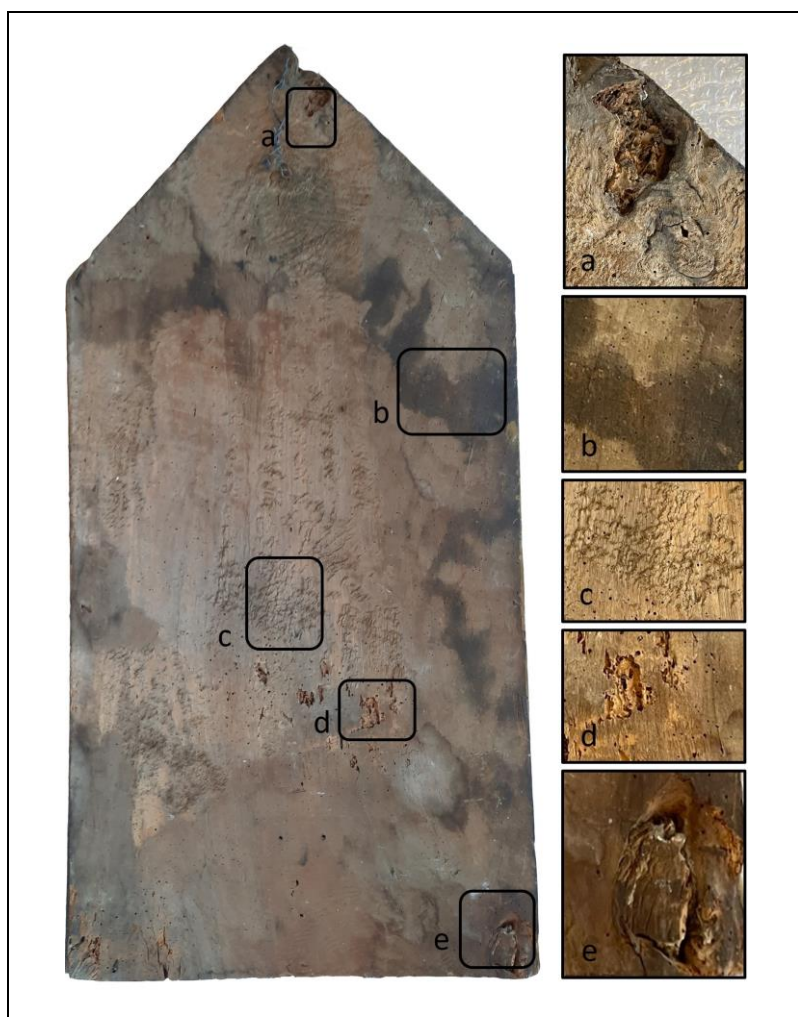
Figure 2. Rear of the wooden support. Details of the observed defects: (a) and (e) - knots, (b) discoloration, (c) truncated fibres, (d) damage caused by entomatic galleries.
