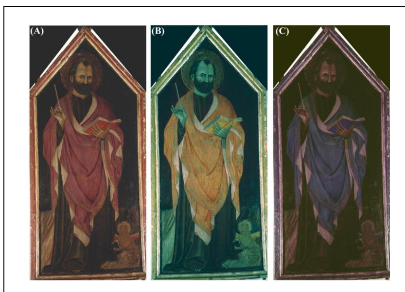
Figure 7. HMI images of the painting: (A) RGB calibrate image; (B) IRFC and (C) UVFC images.
