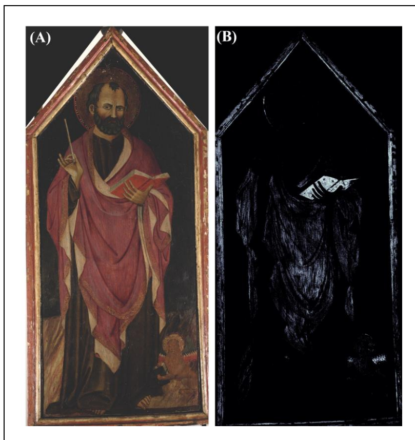
Figure 8. HMI images of the painting: (A) RGB calibrate image, (B) result of the chromatic similarity algorithm.
